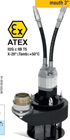
**SP36 ATEX** is a 3" hydraulic waste pump for clear and heavily loaded liquids, impeller and shell are made in stainless steel. The pump produce high performance thanks to hydraulic power and the exclusive closed single channel impeller which allows very high efficiency with flow rates up to 1600 L / min, head up to 50 meters.
