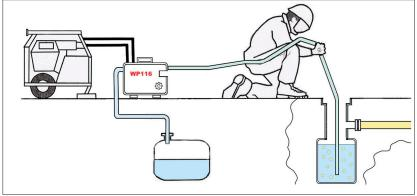
WARNING The pump must not run completely dry for more than two minutes, this could damage the seals, if there is water in the siphon the pump will stick and pump after a few seconds. The pump can tolerate partially dry uses, as long as there is a minimum presence of water due to a small loss from a district heating network. A couple of minutes after the complete complete evacuation of the water must be interrupted.
